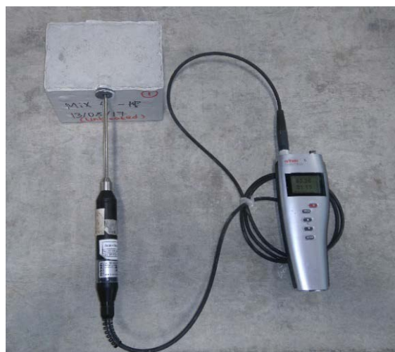
Figure 3-19: Relative humidity measurement setup
