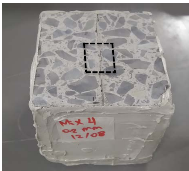
Figure 3-17: Chloride profiling method (cracked concrete)
