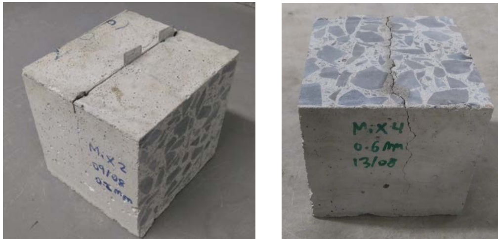
Figure 3-7: Before and after removal of top concrete layer
