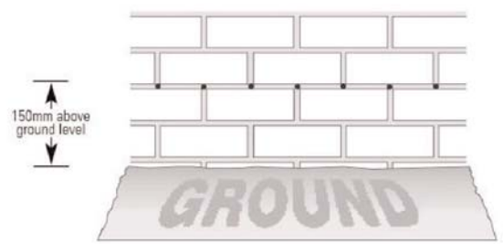
Drilling pattern for Stretching Bond
