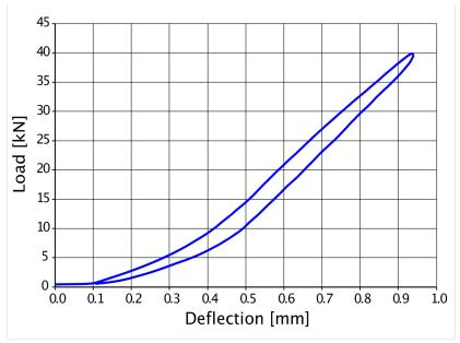
Static stiffness determined analogously to DIN 45673-1. Test specimen dimensions  $1000 \times 180 \times 25 \text{ mm}$ .
