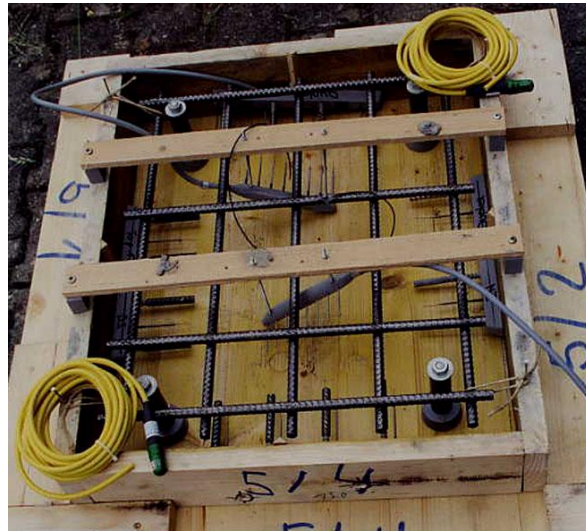
Fig. 2. Instrumentation and reinforcement bars and grid embedded into the concrete plates (see text for explanation). The steel grid is positioned in the rear (wall) side of the plate.
