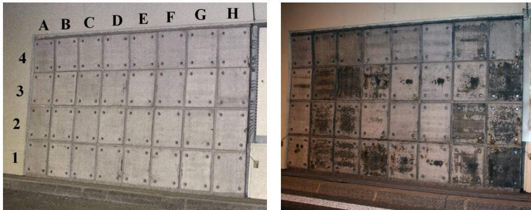
Fig. 1. Visual state of test panels in Naxberg tunnel in year 2000 (left) and 2012 (right).
