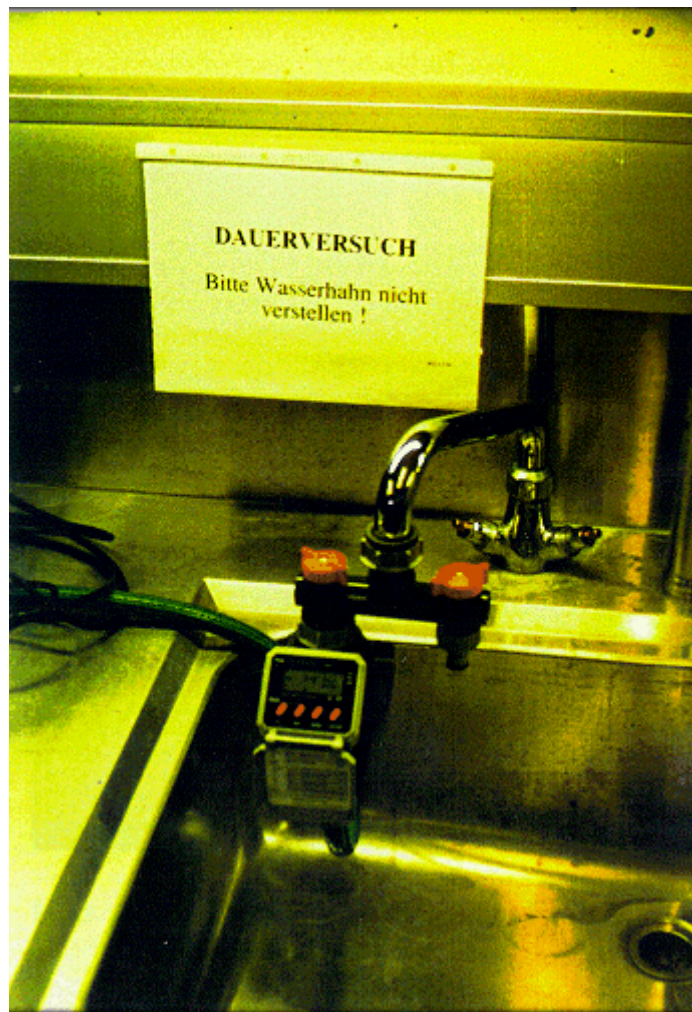
Photo 3 Timer to control spraying
