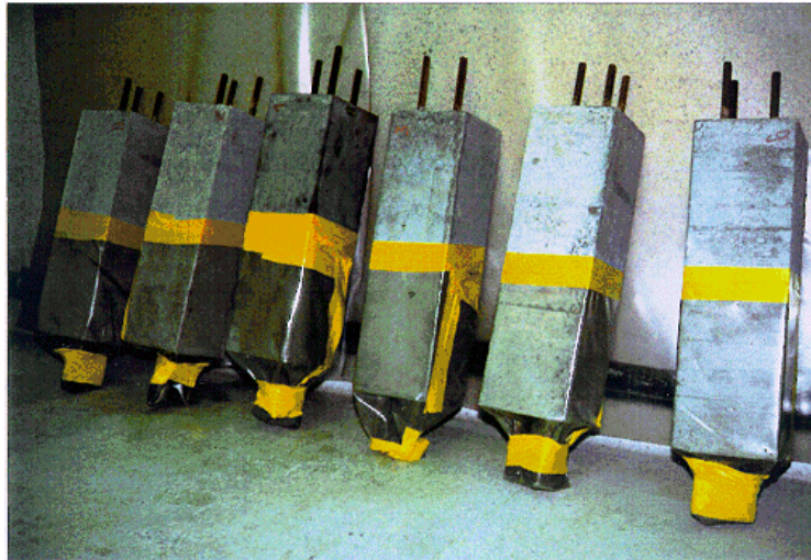
Photo 4 Application of FerroGard-903 on one side of specimens
