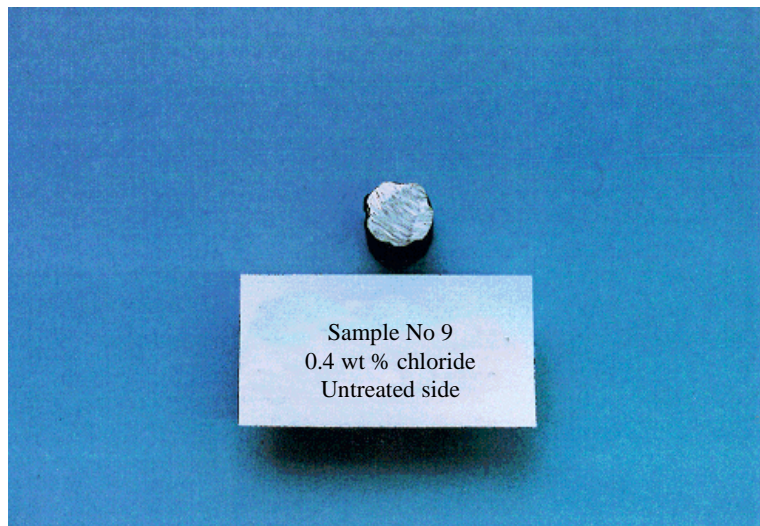
Photo 6 Bright steel cross-sectional area of sample No. 9, untreated side
