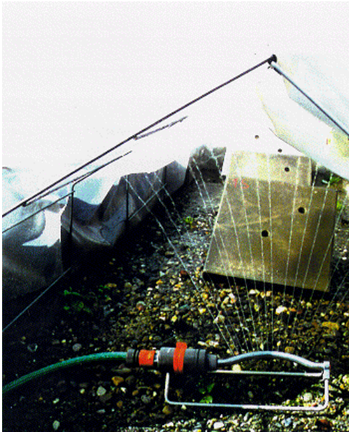
Photo 2 Accelerated weathering by defined spraying of specimens
