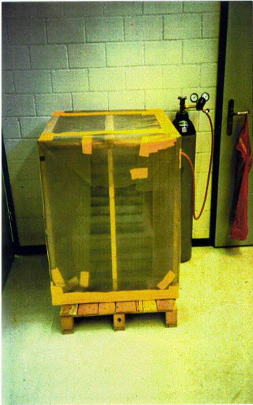
Photo 1 Accelerated carbonation in a CO 2 rich atmosphere
