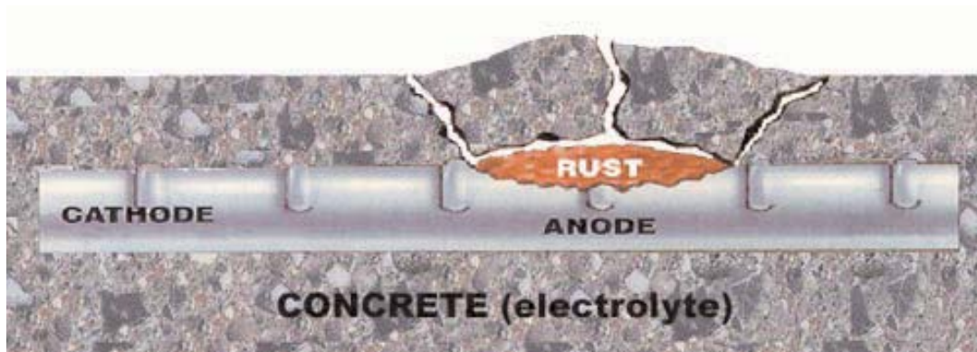
Figure 2: Formation of rust causing spalling of concrete
