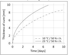
Diagram 1: Curing speed SikaTack® DRIVE (60min)
