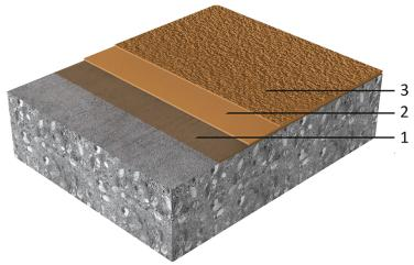
Sikafloor® Pronto RB-25 system (~3–5 mm) / Application on horizontal surfaces
