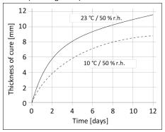
Diagram 1: Curing speed Sikaflex®-212 FC
