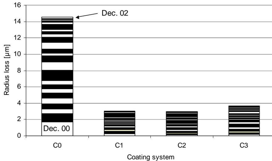
**Figure 4:** Average cumulative radius losses of steel sections in three buildings in the 25 month monitoring period
