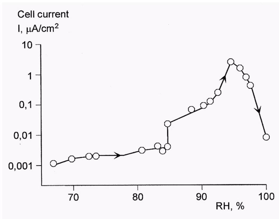
**Figure 1:** Relationship between cell current and relative humidity in concrete according to [2]
