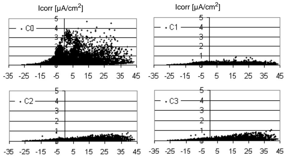
**Figure 5:** Instantaneous corrosion currents plotted against the temperature of the concrete at the moment of measurement. The horizontal axes represent temperature in  $^{\circ}\text{C}$  and vertical axes corrosion current in  $\mu\text{A}/\text{cm}^2$
