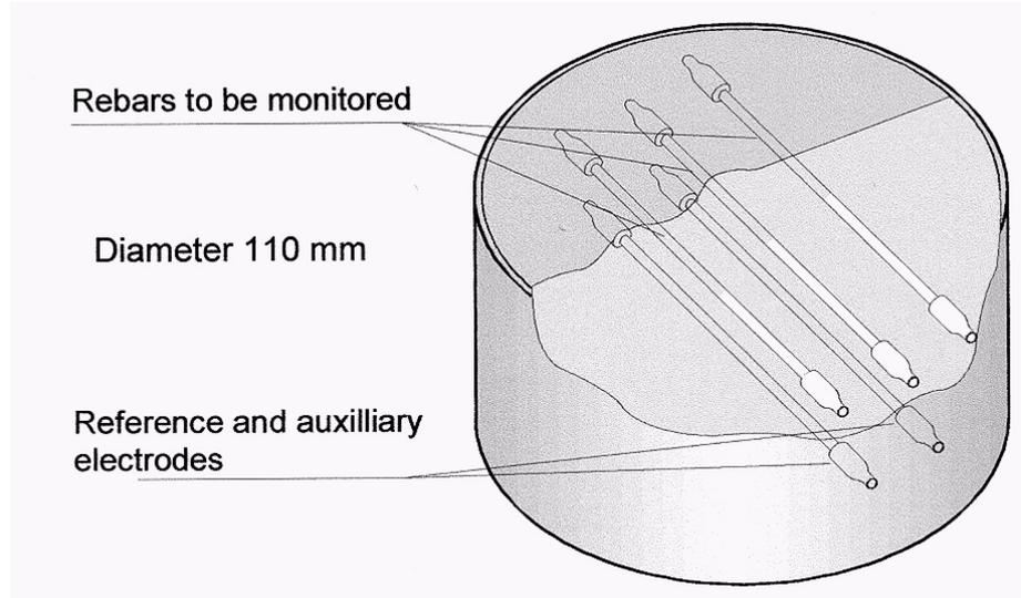
**Figure 2:** Schematic diagram of the sensor developed
