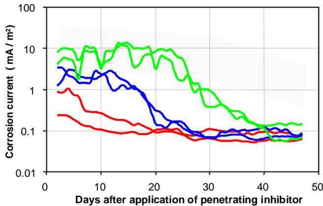
Fig. 4: 75.4 MPa concrete: Change in corrosion current with time after application of Sika FerroGard-903
