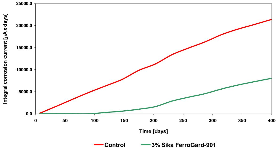
Fig. 2 Cracked concrete beam corrosion test: Integral corrosion current vs. time
