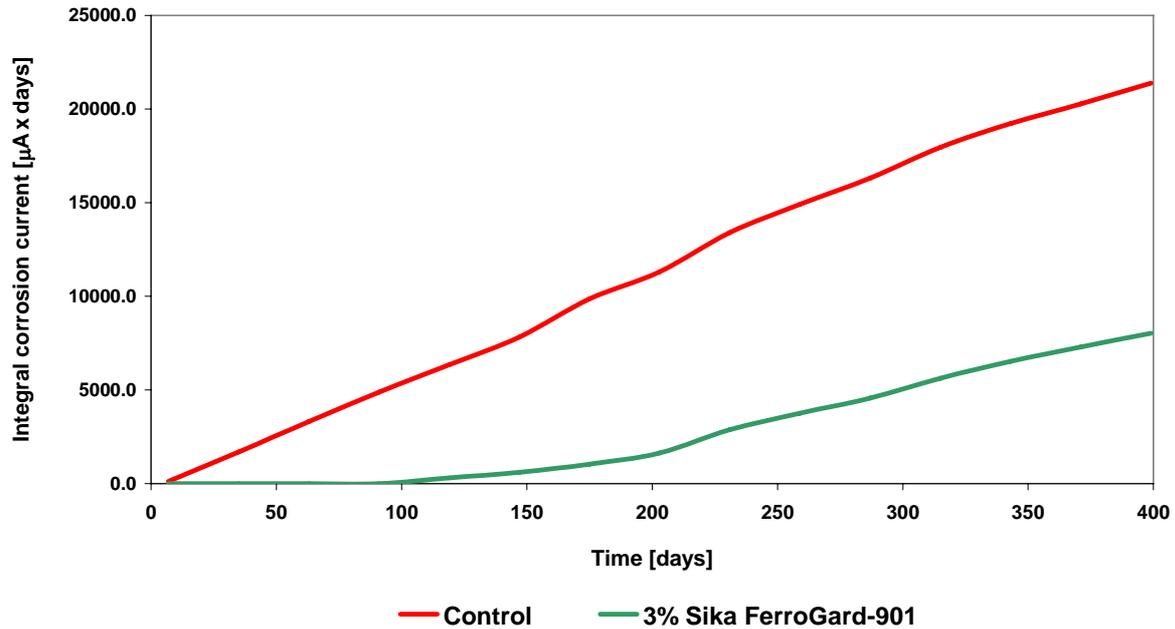
Fig. 2 Cracked concrete beam corrosion test: Integral corrosion current vs. time
