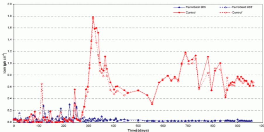
Fig. 5: Change in measured corrosion current density ( $I_{corr}$ ) for Sika FerroGard-903 treated and control concrete specimens exposed to an accelerated chloride ponding procedure.
