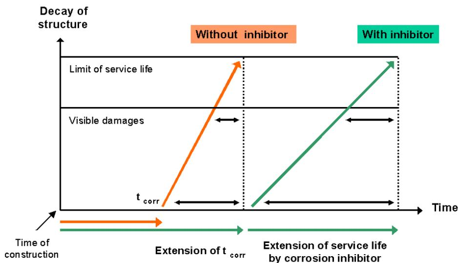
Fig. 6 Extension of service life of steel reinforced concrete structures by corrosion inhibitors
