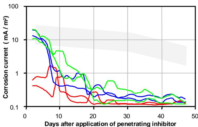
Fig. 3 and Fig. 4: Specimens treated with Sika FerroGard-903: Curves for 10 mm concrete coverage are shown in green, for 20 mm in blue and for 40 mm in red. Control samples: Range of measured corrosion currents for 10, 20 and 40 mm concrete cover shown as hatched area.
