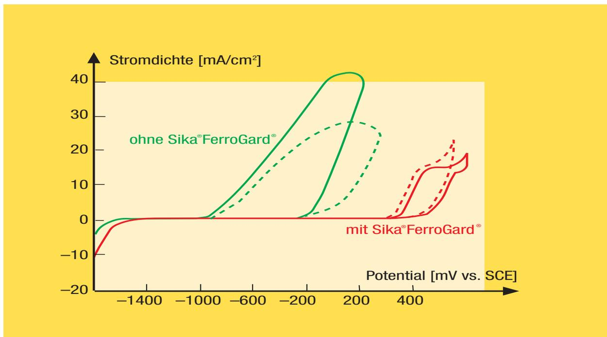
Fig. 1 Potentiodynamic polarisation on mild steel in alkaline solutions containing chloride ions
