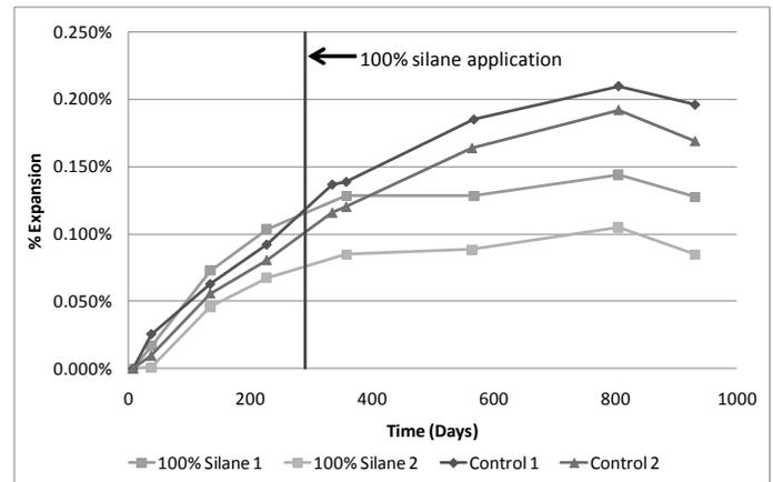
Figure 8. Expansions for 100% silane-treated and control RCA bridge decks.
