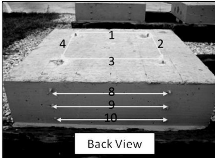
Figure 6. Expansion measurement locations on bridge deck specimen. A similar arrangement was used for the slabs. (Bentivegna 2009).
