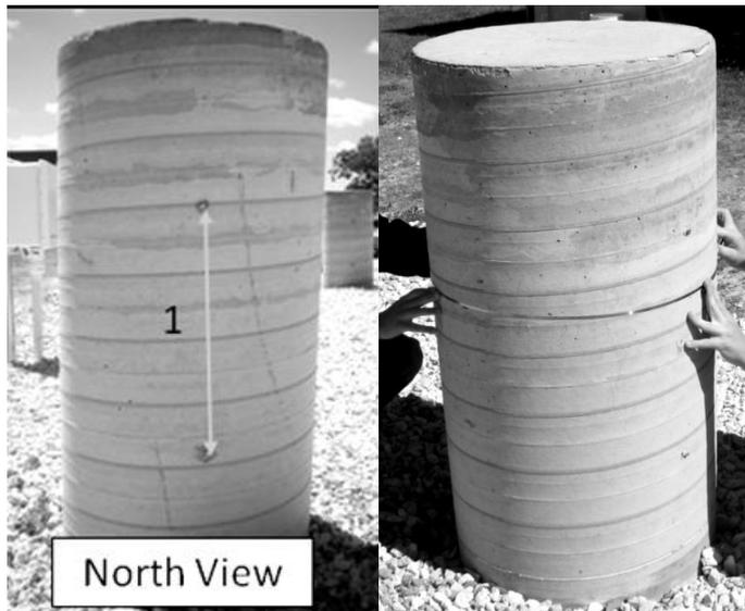
Figure 7. Column expansion measurements. 500 mm vertical gauge length (left) and circumference measurement (right). (Bentivegna 2009).
