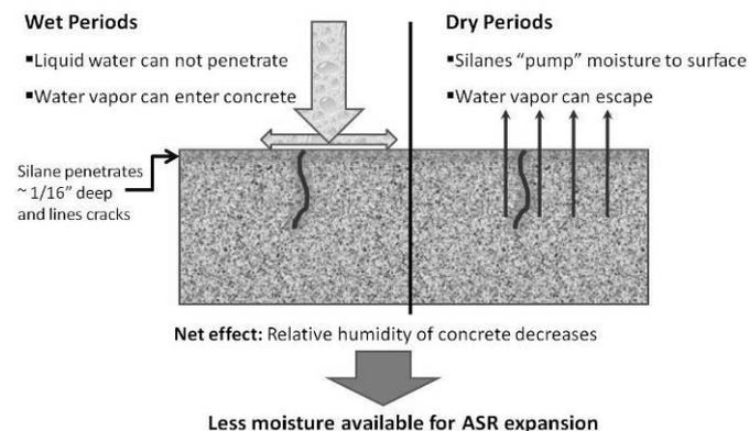
Figure 1. Mechanism of silanes.
