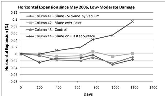
Figure 5. Horizontal expansion, low-moderate damage columns.
