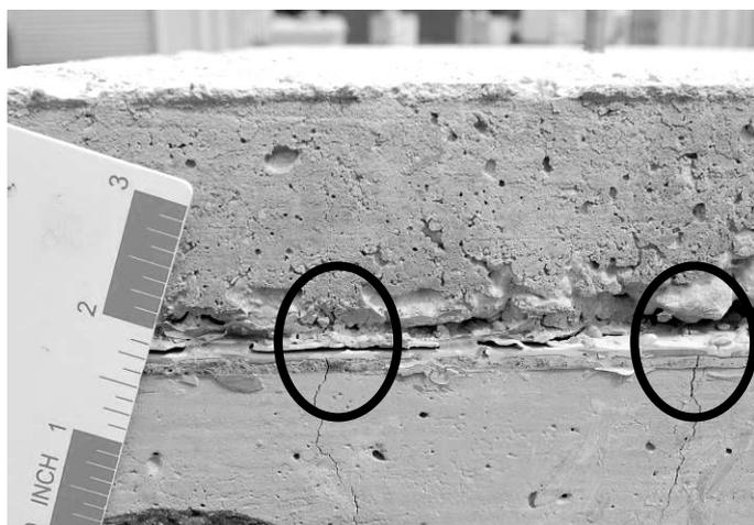
Figure 9. Cracks (circled) in substrate concrete extending into the first layer of Membrane 1 on RFA bridge deck.
