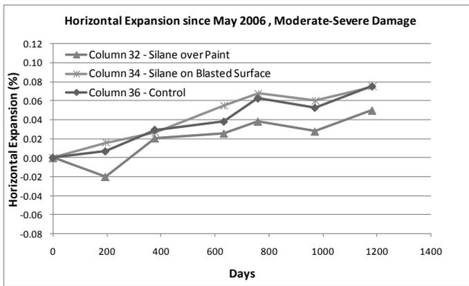
Figure 4. Horizontal expansion, moderate-severe damage columns.
