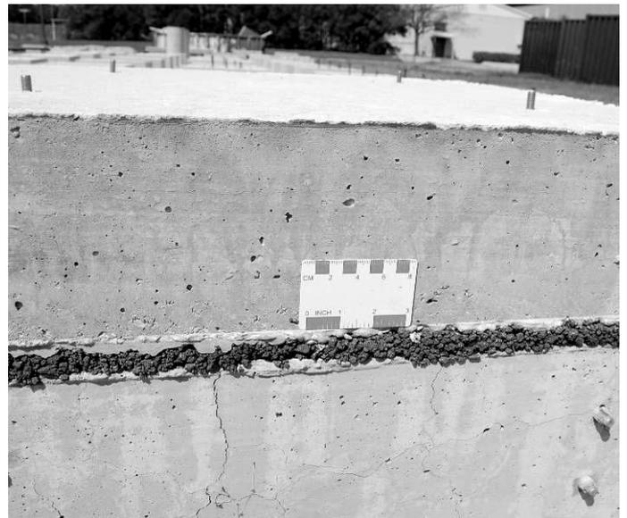
Figure 11. RFA slab with 300 mm concrete overlay and 25 mm asphalt debonding layer.
