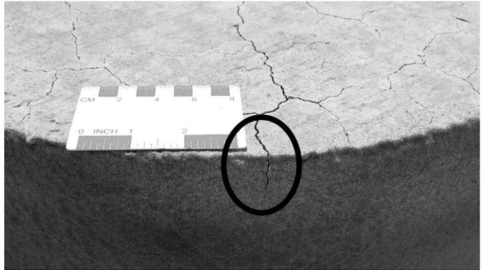
Figure 10. Crack (circled) that has passed completely through Membrane 1 on an RFA column.
