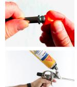
4. Apply the flat nozzle to the end of the Spray Application Gun.
