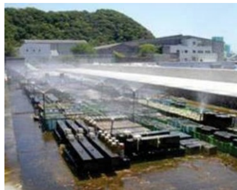
Fig. 3: Test site for salt spray exposure testing at the Kagoshima University in Japan.
