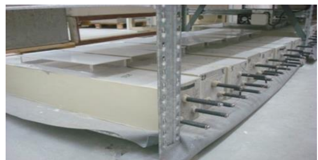
Fig. 1: Prepared concrete beams for corrosion testing.
